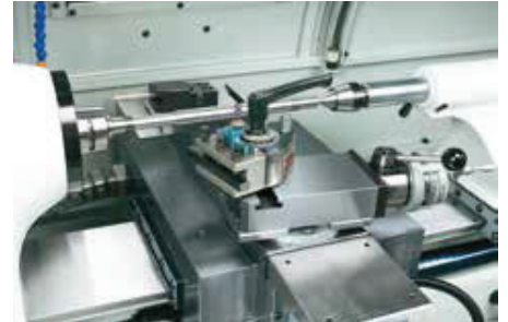
Lathe center in tailstock single tool on quick change tool holder on compound slide.
