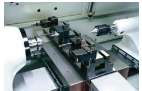
Multiple "single" gang tool blocks each holding a single tool holder.
